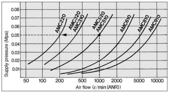
How to view the diagram: If the AMC510 is operated at a flow volume of 1000 //min (ANR), the supply pressure will be 0.05MPa.
