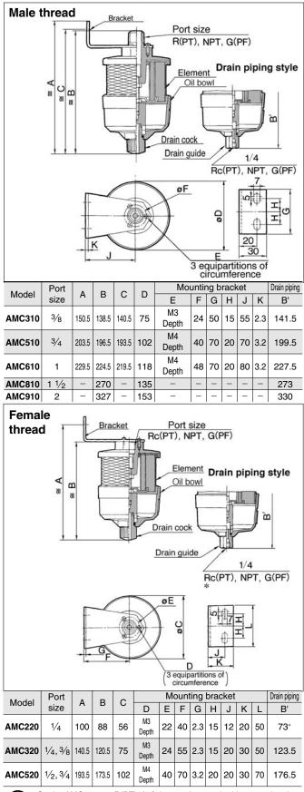
\* On the AMC220, an R(PT)1/4 fitting can be attached by removing the drain cock.
